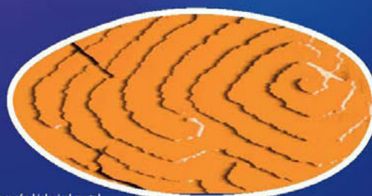
Surface of a biological crystal showing stacking faults as seen by atomic force microscopy . © IUCr - journals
