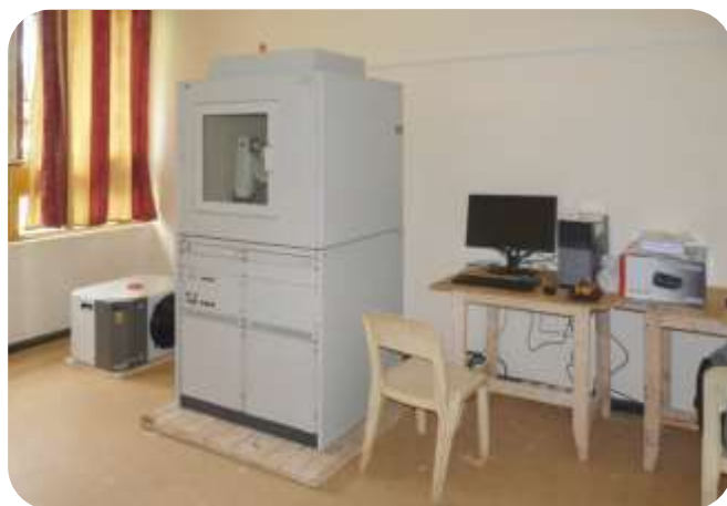
D5005 powder diffractometer installed in Dschang
