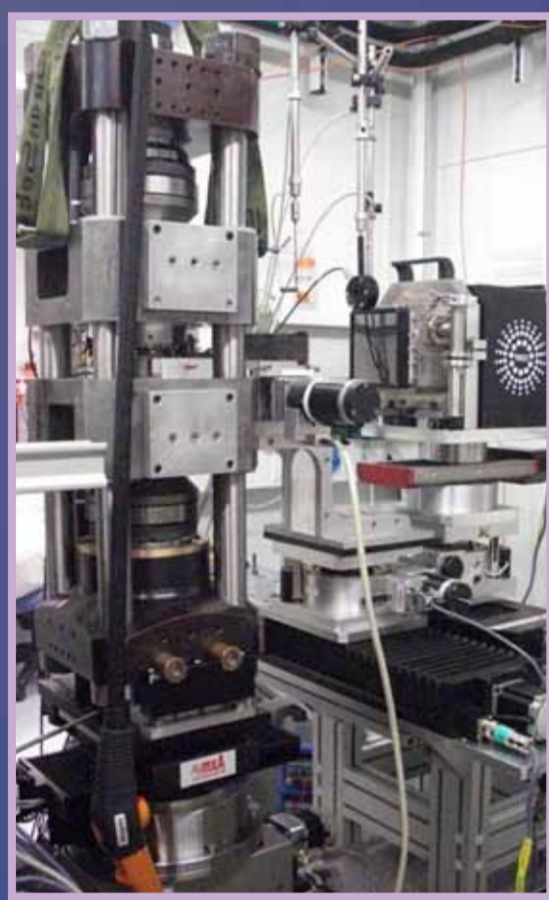
Although high pressure set-up can be very large, the pressure is inevitably lower in experiments with larger anvil cells (few mm). Source: RotoPEC-IMPIC & ESRF
